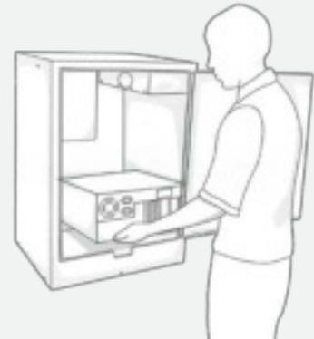
3. Cables entering or exiting the enclosure pass through a cable port, usually located on the back of the enclosure. If your cable ports came with a rubber grommet, simply use a utility knife to make two small incisions: creating the shape of an 'X' or '+' and run the cables through the space.
