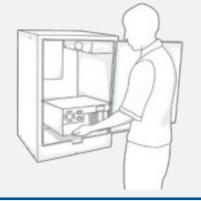
**3.** Cables entering or exiting the enclosure pass through a cable port, usually located on the back of the enclosure. If your cable ports came with a rubber grommet, simply use a utility knife to make two small incisions: creating the shape of an 'X' or '+' and run the cables through the space.
